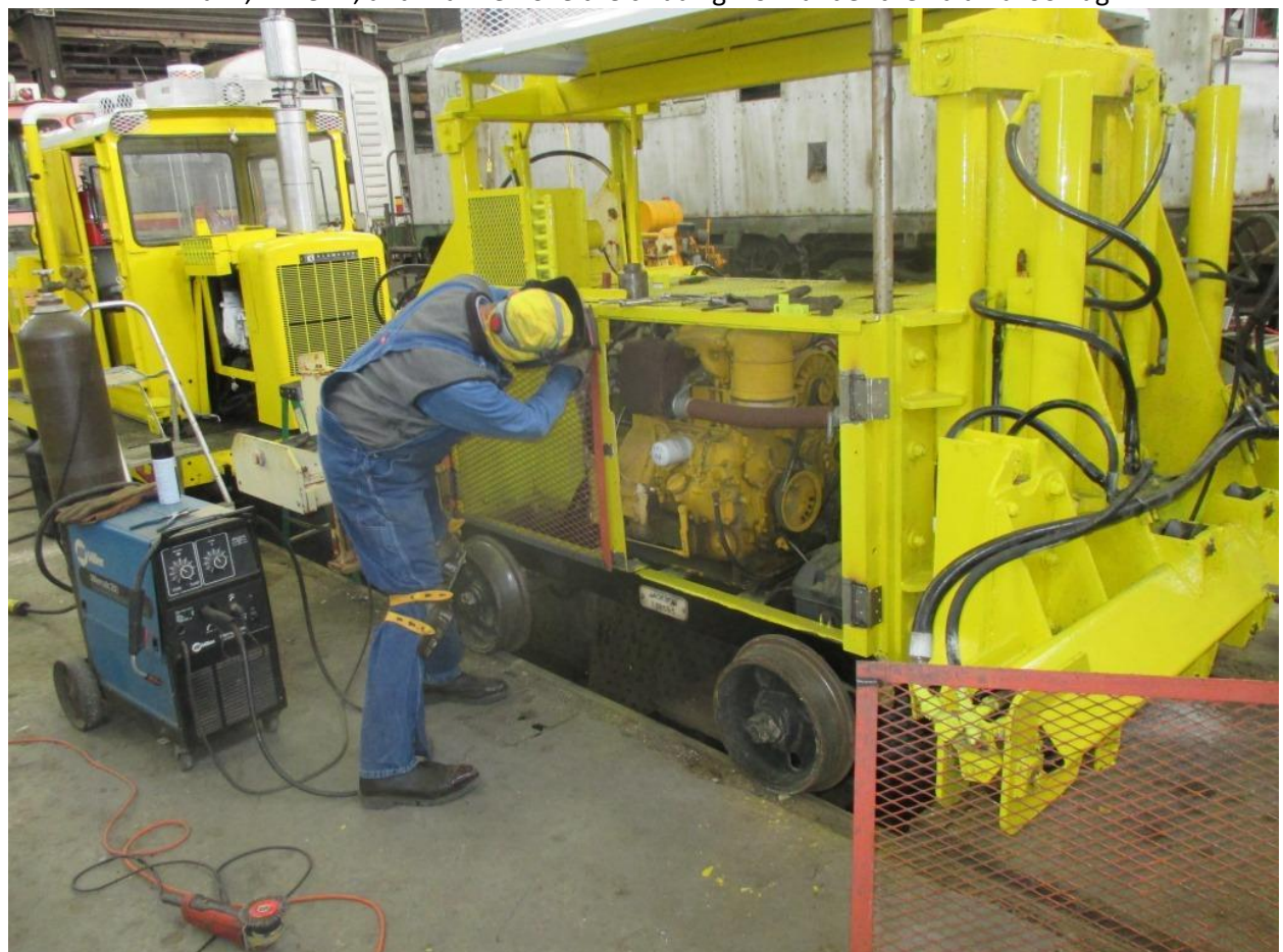
Cliff installs new security doors over the engine compartment of the Jackson 125 Tie Exchanger
